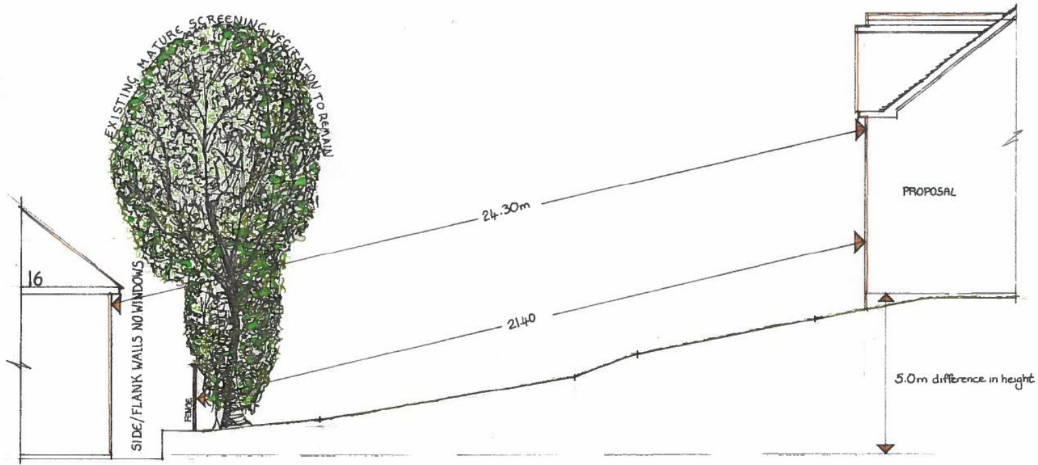
SECTION ILLUSTRATION SHOWING RELATIONSHIP BETWEEN PROPOSAL & No. 16 THE BADGERS & HOW SEPARATION DISTANCES EXCEED REQUIREMENTS & THE EXTENT & SCALE OF THE INTERVENING MATURE SCREENING 1:100
